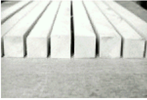
Pic. 1 End grain of each piece should not slant the same way, they should alternate //\\//\\//\\
