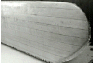
Pic. 11 Drape cloth over board that suspended by two wires, each wire is attached to a finishing nail, one in the end of tip the other in the top of head. Paint on the epoxy wetting out all of the cloth. Squeegee off all excess until it starts to look dry (no thick shiny pools of epoxy). Allow to harden. Trim off excess fiberglass with utility knife or large scissors. Block sand to remove high spots, (80 or 100 grit OK) try not to sand into fiberglass. Lay board on side, keep it level with shims under tip and trailing edge. Apply final coat of epoxy allow to harden, then do other side. Block sand again filling any low spots with dab of epoxy or glazing putty, wet sand with 180 grit or 220. You can paint it if you like. There is so-called epoxy paint in spray cans, which is used on cloths washers and drier appliances. I decided to not paint my board, I was anxious to use it and I wont have to touch up any paint chips. I finished it off with a good wet sanding using 400 grit on a soft rubber block.
