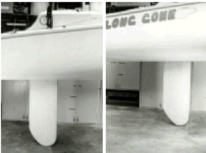
Pic. 12&13 Finished product. Test for minimum side play, grab end of board and move side to side. If there is to much side play, shim up head with small strips of fiberglass and epoxy, board should go up and down smoothly with some resistance.
