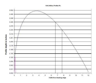
The plot shows the calculated foil shape using exaggerated elevation to make it easier to read values from the plot. The dimensions are in inches.
