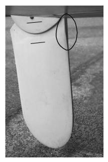
The third problem is that the two "cheeks" which form part of the rudder joint extend unnecessarily far down into the immersed flow, providing an additional source of turbulence and drag.
