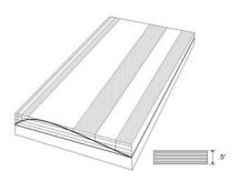
Marking the stripes on the surface is futile, since these markings will be sanded off. But by marking them on some wood on either side, you can use a straight edge for a quick check whether you have sanded deep enough. I kept the rudder head attached as I was shaping the foil. That gave me a nice flat area to clamp my work piece and to mark these locations.
