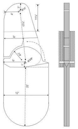
material, and add two separate pieces for the "cheeks" of the rudder joint. As material I decided to use 2 sheets of .5" plywood, glued back to back, which would give me 1" at maximum thickness. After shaping it, I planned to epoxy seal the wood and cover it with a thin layer of glass cloth for protection.
