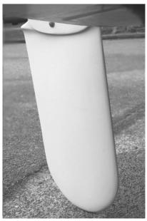
At this stage, after letting the epoxy cure for a few days and sanding smooth the area of the rudder joint, I drilled and reinforced the holes for the rudder and tiller bolts. The rudder bolt is a 3/8<sup>°</sup> carriage bolt. I epoxied a nylon bushing in one cheek, and filed the hole in the other cheek to a square, which I reinforced with epoxy. The tiller bolt also got a nylon bushing.
