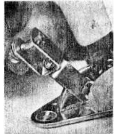
Attach bow swivel shackle to forward clevis pin and keeper ring.
