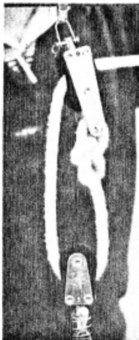
Tie one end of the mainsheet to the becket, pass the other end of the line through the block on traveler from fore to aft up through the block on the end of boom from aft to forward.
